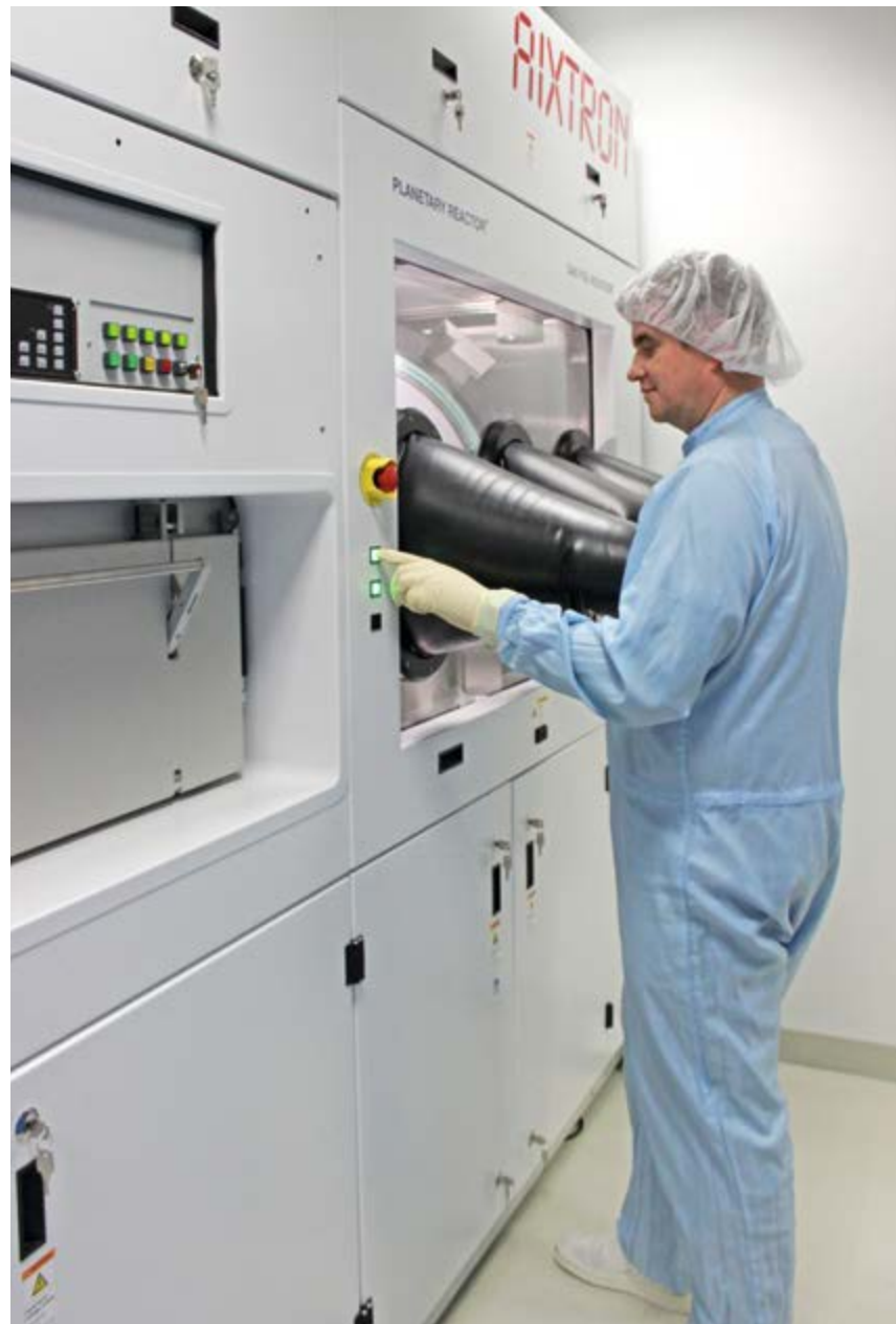
MOVPE reactor for growth of GaAs-based devices.
