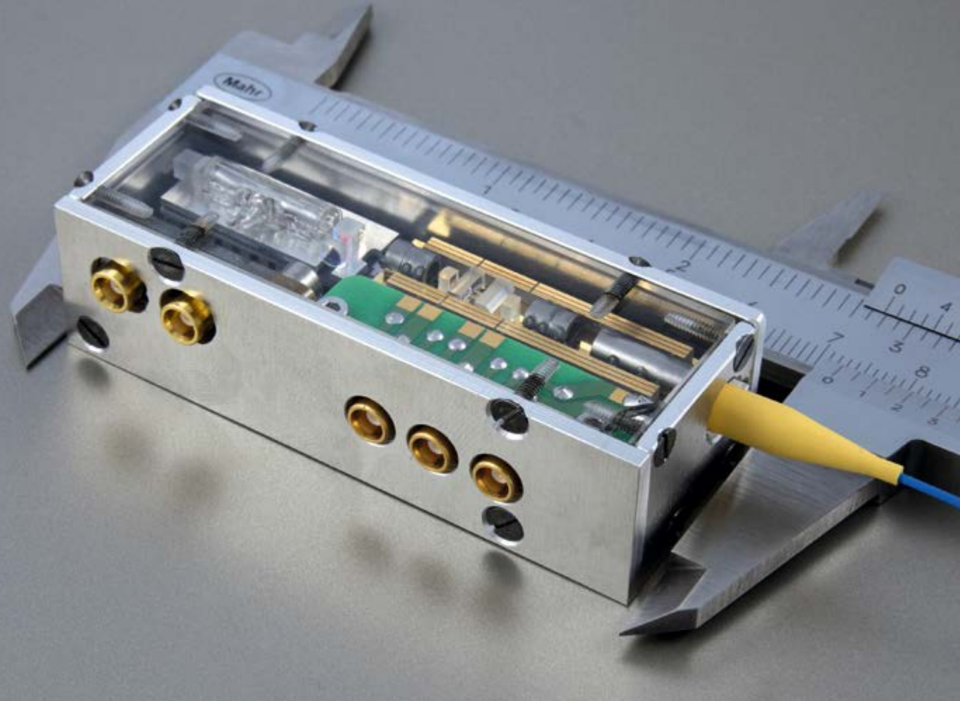
Fig. 1. Optical frequency reference module developed within the IQSoC project.
