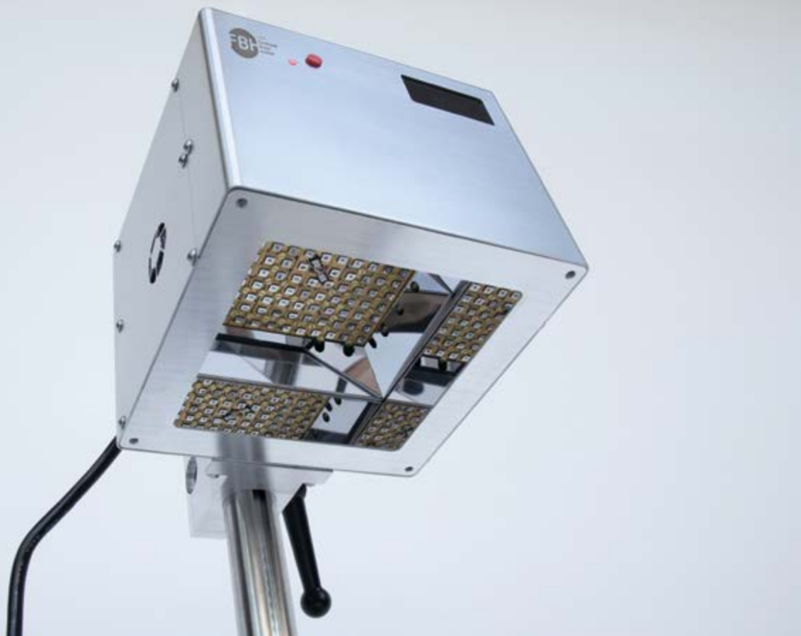
Fig. 1. UV LED irradiation system where the radiation unit with the 120 far-UVC LEDs and the vertical and slanted reflectors are visible.
