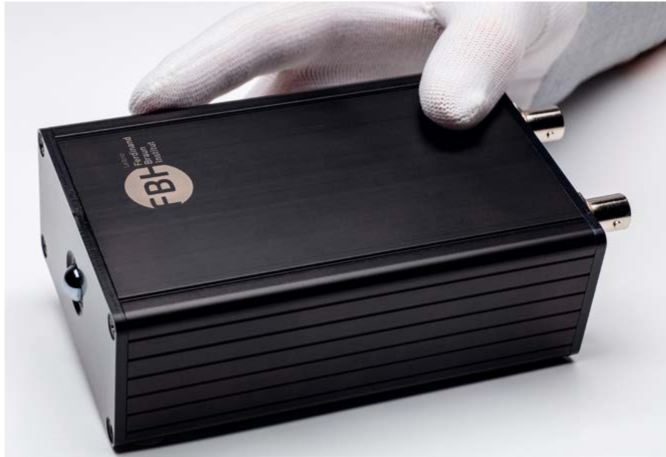
Fig. 1. Single THz detector with electronics ready to use for customers.
