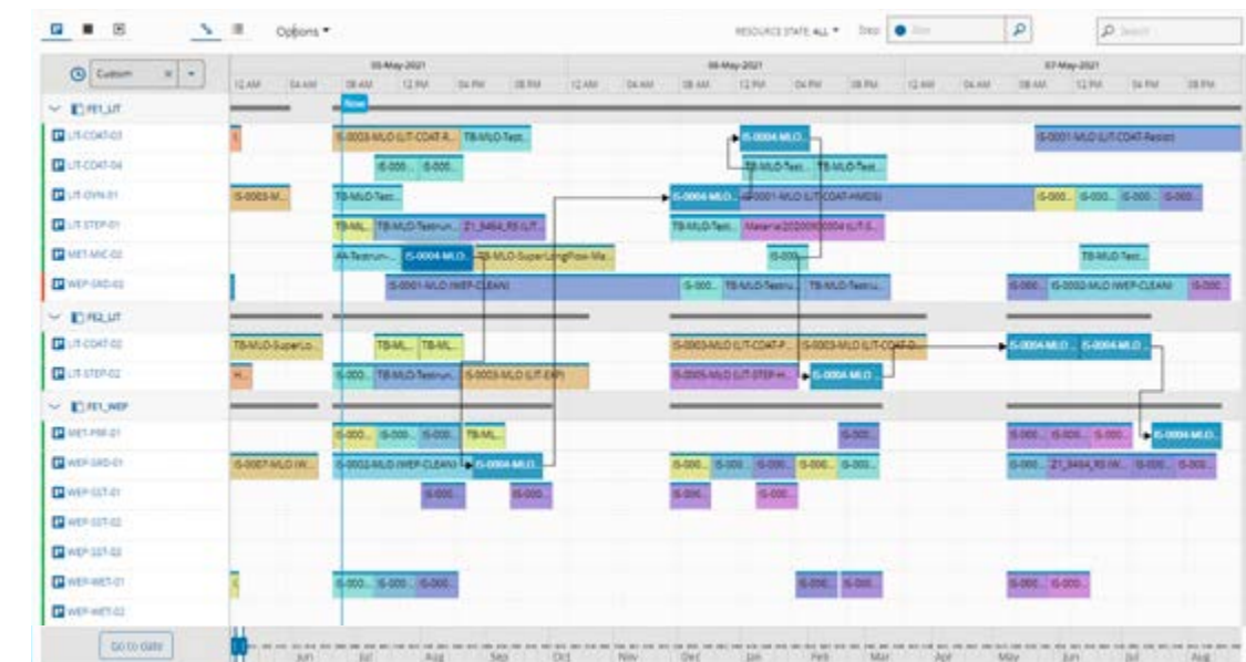
Fig. 2. Gantt chart showing process flows of materials (symbolized by colored boxes) across various process resources (listed in left column). The MES computes various planning scenarios that optimize various performance indicators such as resource utilization, fastest overall production delivery, minimization of average processing time or deviation from delivery dates and many more.
